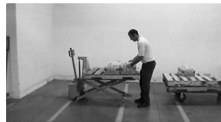
Figure 4. Scissors lifts pallet jacks are an example of an ergonomic solution that could maintain lifting between knee and waist height.
